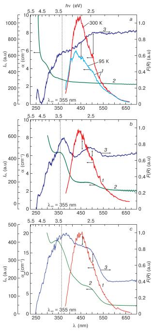
**Figure 4.** (1) IPL luminescence, (2) absorption R and (3) Kubelka–Munk function F(R) spectra for LGT crystals grown in different atmospheres: (a) Ar; (b) Ar + 0.5 % O<sub>2</sub>; (c) Ar + 2 % O<sub>2</sub>.
