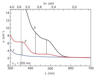
**Figure 3.** Luminescence spectra of LGT crystals grown in different atmospheres: (1) Ar; (2) Ar + 0.5 % O<sub>2</sub>; (3) Ar + 2 % O<sub>2</sub>.
