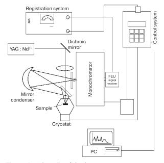
Figure 1. Schematic of luminescence spectrum measurement setup.
