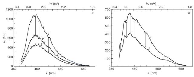
**Figure 2.**  $\lambda_{ex} = 355$  nm luminescence spectra of LGT crystals grown in different atmospheres for (*a*) 300 and (*b*) 95 K. *a*: (*1*) Ar; (*2*) Ar + 0.5 % O<sub>2</sub>; (*3*) Ar + 2 % O<sub>2</sub>; *b*: (*1*) Ar; (*2*) Ar + 2 % O<sub>2</sub>.
